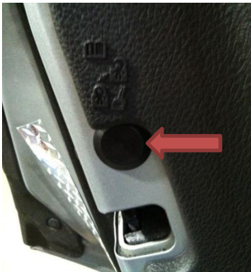
Child safety lock adjustment is located under black rubber plug in picture to the left.
