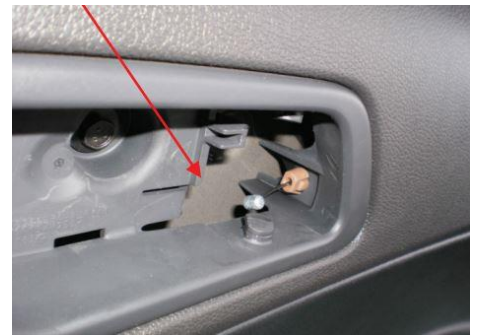
Above is a picture of a broken handle with cable easily accessible.
